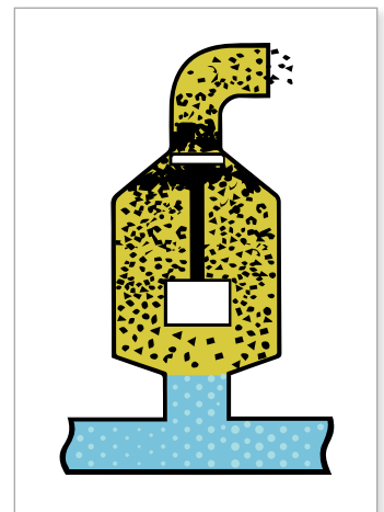
Negative flow rubbish 'bird nest' caught in valve. Blocked and/or leaking
